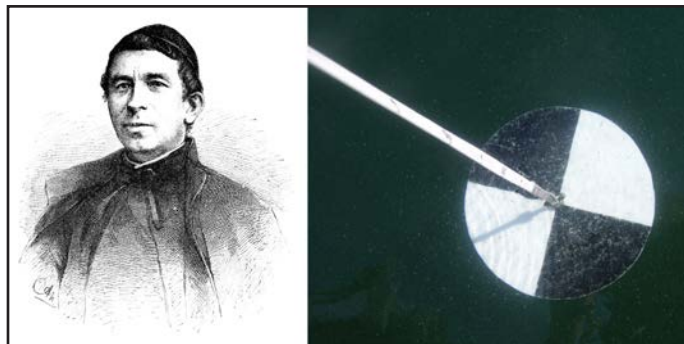
The Italian astronomer, Angelo Secchi (1818-178), and the limnological tool named after him. Secchi initially developed the disk to measure the depths of Venetian Canals
