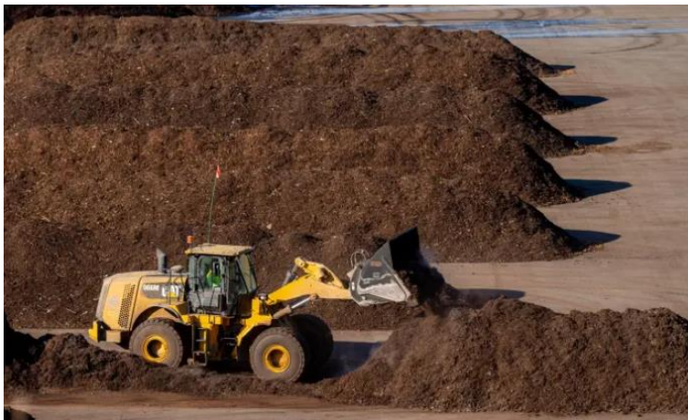
Figure 3-4 Example of Front-end Loader Managed Windrow
